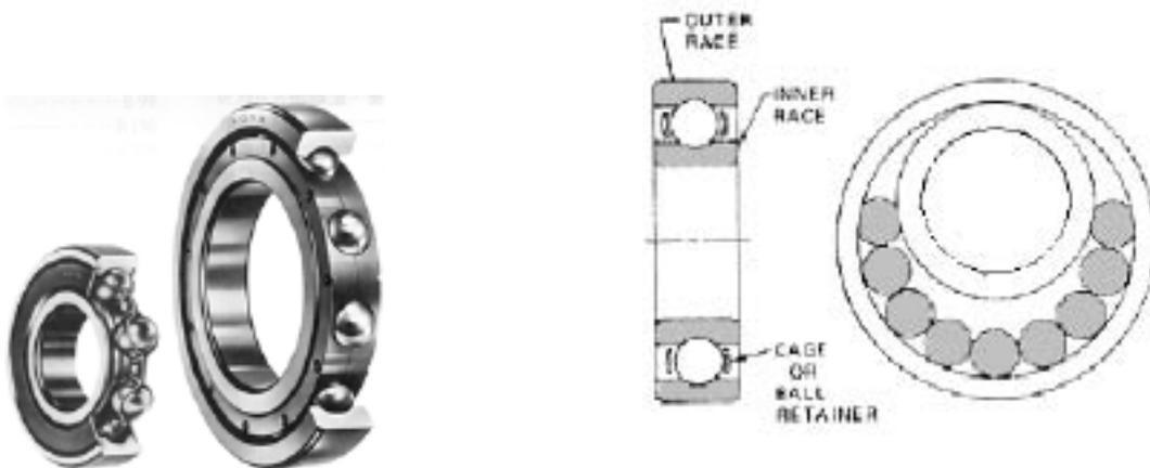
These are sometimes called Conrad bearings. They are assembled by offsetting eccentrically the inner and outer rings to allow the insertion of balls (see figure above). The Conrad bearings therefore have uninterrupted ringways (no filling slot) which permits excellent bearing performance under light to moderate radial loads, relatively moderate axial loads, or combined radial and axial loads.
