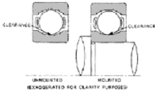
Radial ball bearings are usually supplied with a specified radial clearance, which will normally diminish during mounting because of interference fits with the shaft and house. After mounting, the bearing should have a small radial clearance remaining.
