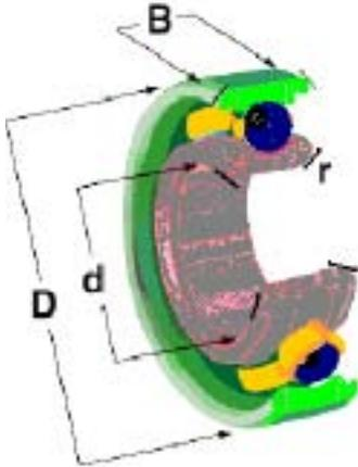
Bearing boundary dimensions have been standardized by the international Standards Organization (ISO). Within each diameter series there are several dimension series which are combinations of the diameter series and different width series.
