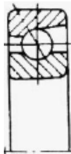
These bearings can be mounted singularly or, when the side surfaces are flush ground, in multiple, either face-to-face or back-to-back for all combinations of thrust and radial loading. Flush ground bearings can also be tandem mounted to permit sharing heavy thrust loads in one direction among two or more bearings.
