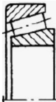
Tapered roller bearings have a high capacity for radial loads, axial loads, and combined loads. The larger the contact angle, the greater the axial load capacity becomes.
