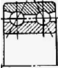
They have the same characteristics as duplex angular contact ball bearings (DB), while having smaller width. They are suited where axial space is limited.
