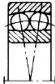
It is a very important consideration in many applications requiring extreme accuracy, at high speeds. Self-aligning ball bearings are recommended for radial loads and moderate thrust loads.
